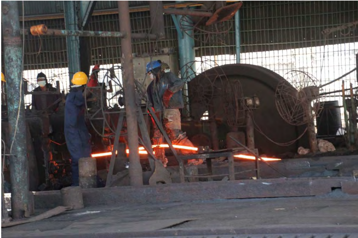
3a: In this work environment workers are exposed to hot items. A proper risk assessment is important to be able to provide the workers with protection from heat; for instance gloves, clothing and shoes (Photo: G.Tjalvin).
