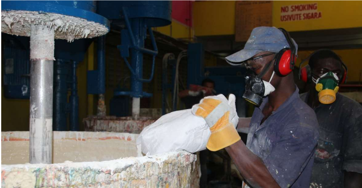
3c: These workers are protected from inhaling chemicals from paint production, as a proper risk assessment has been performed. They have been provided with respiratory protective equipment (Photo: G. Tjalvin).
