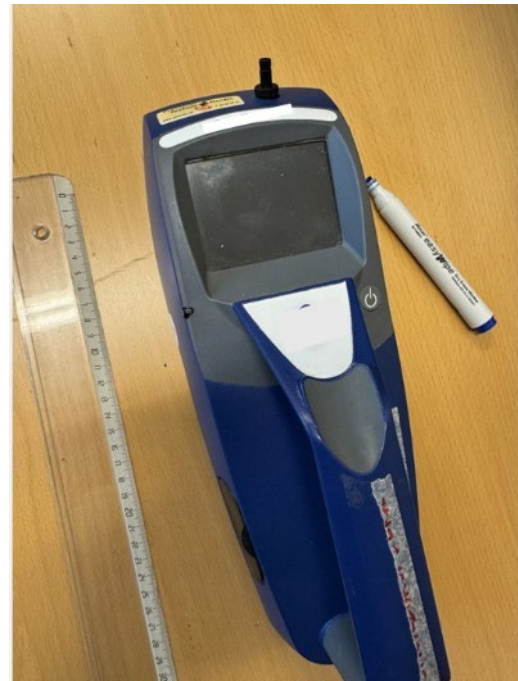
Figure 1.9. Hand-held, direct-indicating instrument for measurement of different particle sizes. ©University of Bergen
