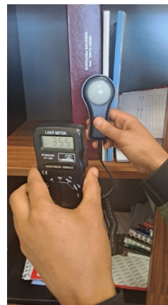
Figure 8.4. The light sensor is placed vertically if the object is read vertically. ©T. Abegaz
