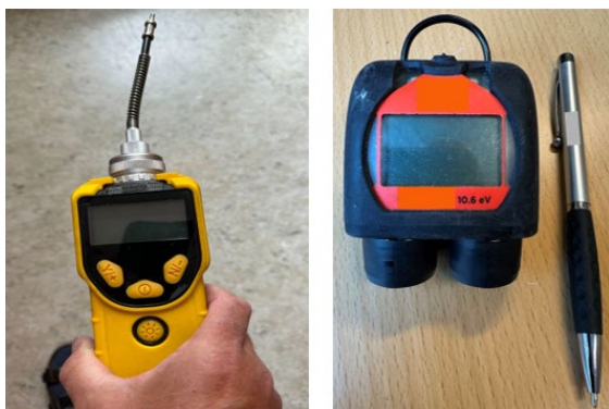
Figure 4.5. Examples of photoionization detection (PID) instruments for measurement of non-specific, volatile organic hydrocarbons (VOCs). A hand-held instrument (left), and a personal monitor (right). ©University of Bergen
