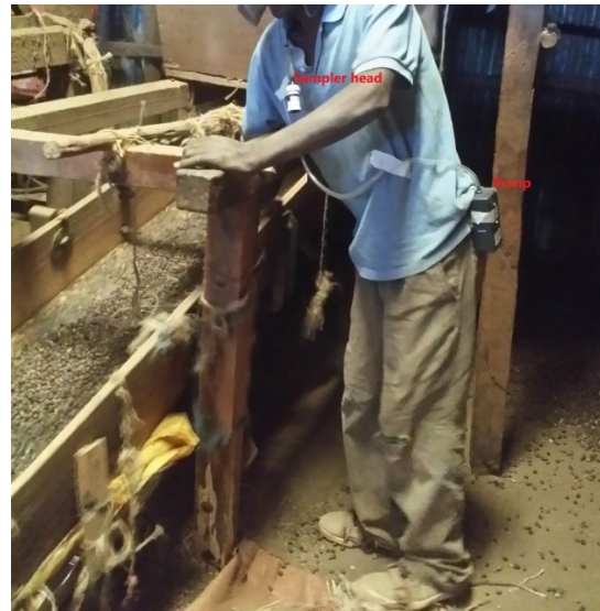
Figure 1.2. Sampling of dust with filtration samplers, showing the location of the sampling head in the respiratory zone of the worker, while the pump is attached to his trousers. ©Samson Wakuma Abaya
