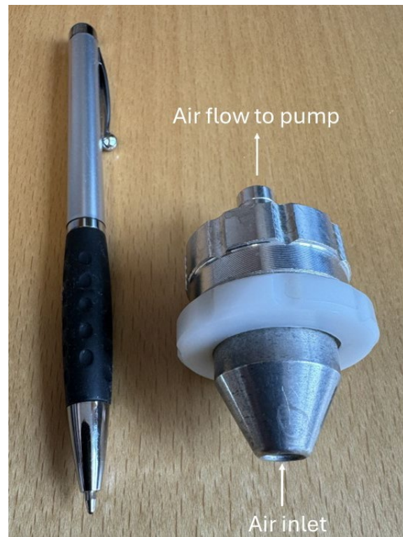
Figure 1.4. The conical inhalable aerosol/dust sampler with filter mounted inside the sampling head. ©University of Bergen
