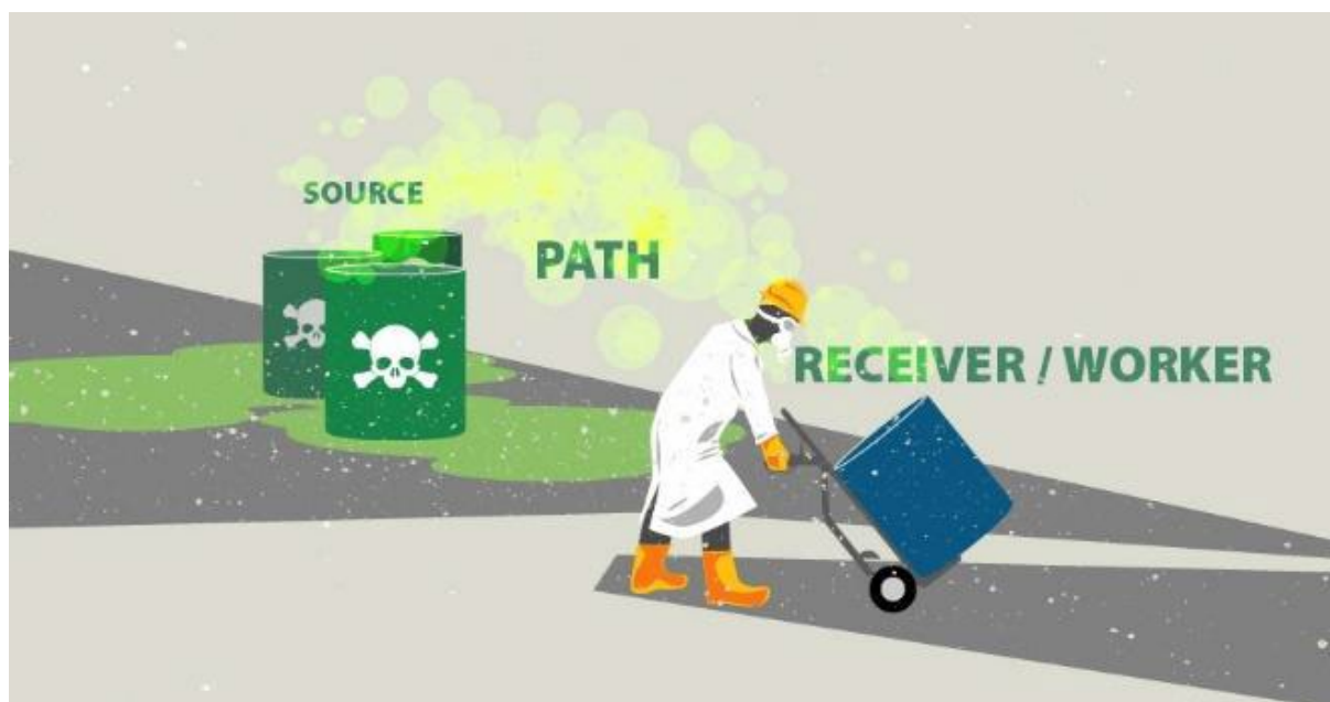
Figure 3. Three main locations of control measures. ©University of Bergen
