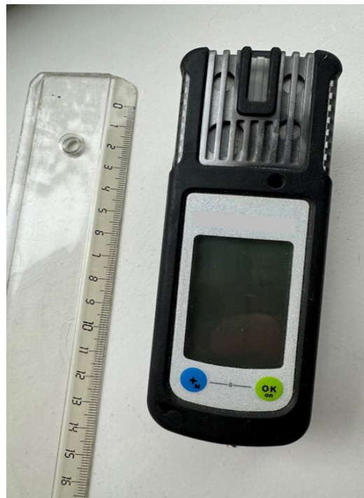
Figure 4.4. Example of an electrochemical sensor for measurement of inorganic gases. ©University of Bergen
