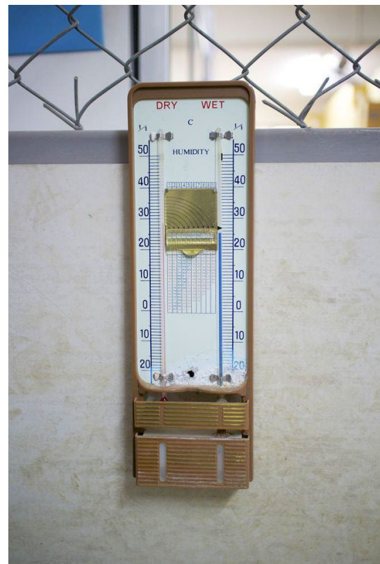
Fig. 6.1. Wet bulb and dry bulb thermometer. © Colourbox
