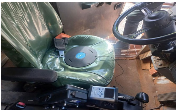
Figure 2.2. Measurement of whole-body vibration using an instrument with an accelerometer inside a seat pad. The seat pad is connected to the computer/logger with a thin wire ©IP Nyarubeli
