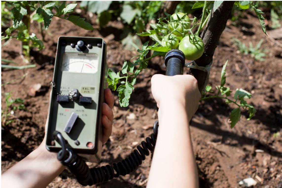
Figure 5.3. The person is using a Geiger-counter to measure the radiation level in the vegetables. ©Colourbox
