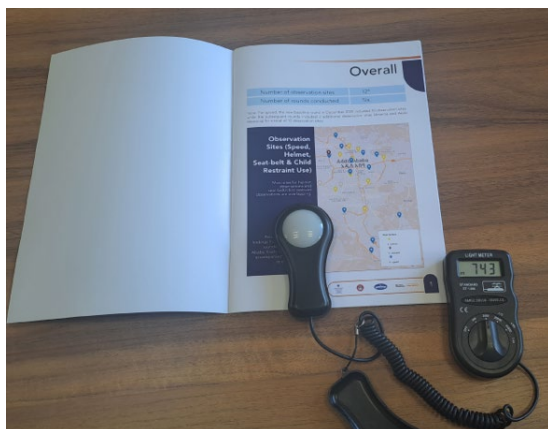
Figure 8.3. The sensor of the light meter placed on the work plane. ©T. Abegaz
