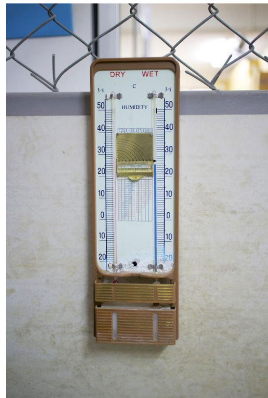
Fig. 6.1. Wet bulb and dry bulb thermometer. © Colourbox
